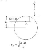
KE + PE (at A) = PE (at B)  $\frac{1}{2}m\left(\frac{2GM}{R}\right) - \frac{GmM}{2R^3}\left[3R^2 - \left(\frac{99}{100}\right)^2 R^2\right]$   $= -\frac{GMm}{(R+h)}$   $\Rightarrow R + h = \frac{2R}{0.0199} \Rightarrow h = 99.5 R$
